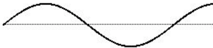
This mode of resonance would be impossible because the string is fixed at each end
