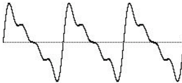
The sum of harmonically related frequencies still repeats at the fundamental frequency
