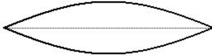
A plucked string vibrating in its fundamental resonant mode
